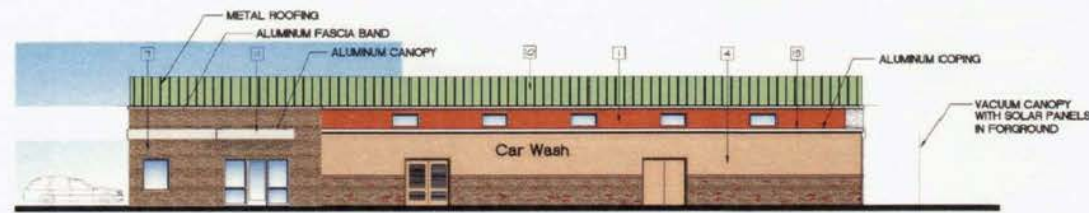
CAR WASH NORTH ELEVATION
